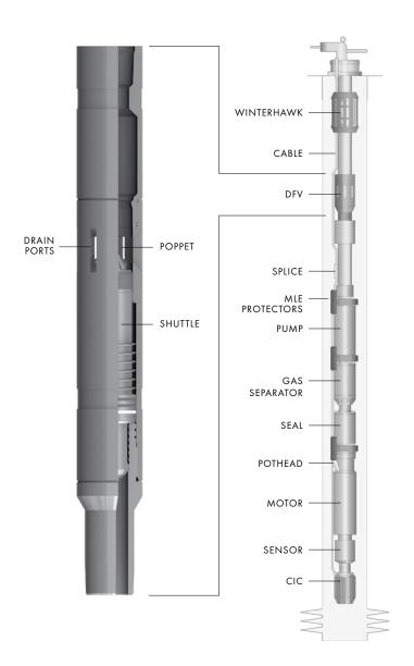
The ESPCT Flow regulated drain and fill valve (DFV) is a tubing mounted downhole tool and it is typically installed in wells requiring drainage of the production tubing upon shut off of the ESP system below it.
